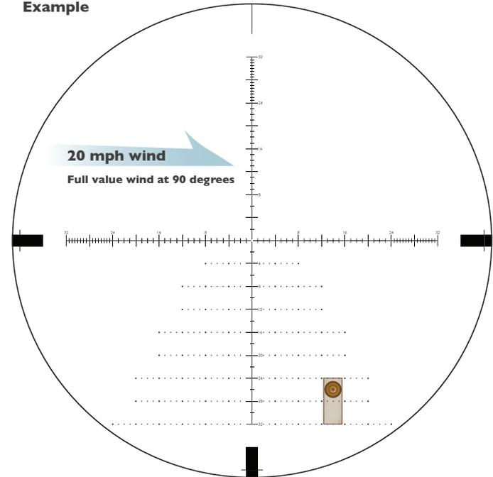
14 MOA reticle windage correction for 20 mph wind at 800 yards using the 26 MOA reticle drop line.
