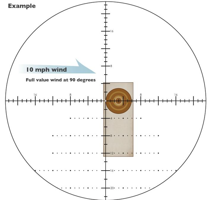
3 MOA reticle windage correction for 400 yard shot in 10 mph crosswind using center crosshair. Elevation adjustment already dialed into riflescope.
