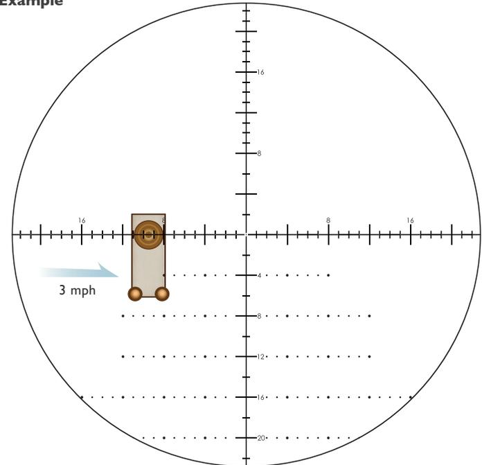
9.5 MOA reticle correction for a target moving at 3 mph at a distance of 800 yards. No wind. Elevation adjustment already dialed into riflescope.
