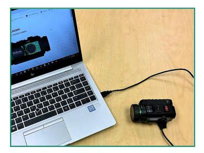
A green light appears and blinks slowly during the charging process. When the battery is fully charged, the light will turn off.
