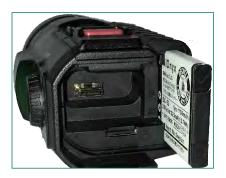
5. Insert the Micro USB cable into the camera USB port.
