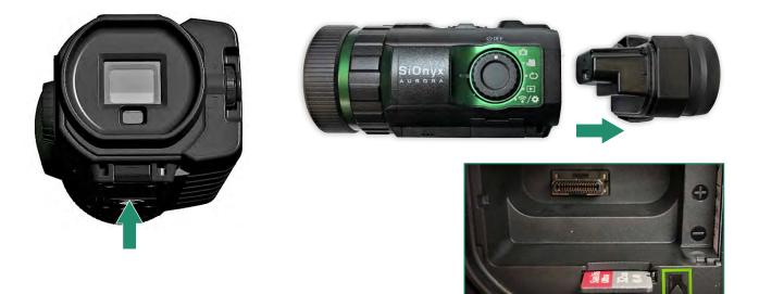
Note: Don't force the SD card into the slot or the data may be damaged.
