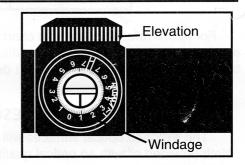
Without disturbing the rifle. adjust windage and elevation screws to center the reticle on target.
