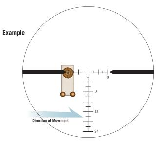
8 MOA reticle correction for a target moving 3 mph at a distance of 800 yards. No wind. Elevation already dialed into turret.
