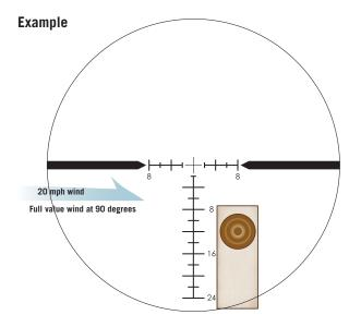
8 MOA reticle windage correction at 500 yards in 20 mph crosswind using 12 MOA reticle drop line.
