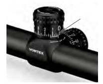
While holding the cap up, rotate dial to reposition the zero mark on the index line.
