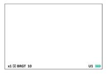
If the light indicator does not light up or blinking and the battery status indicator at the bottom right of the display is not visible or blinking, the battery charging or charging of external power sources must be checked.
