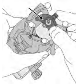
Snap lens spacer into place.
